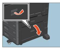
**3** Remove the misfed paper and close the feeder cover.
