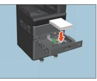
**3** Check that the guide width is correct and there is no folded/curled paper or overloading, and then close the drawer.
