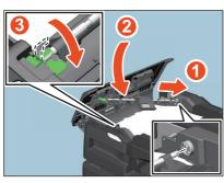
**6** Remove the originals under the original feeder tray.
