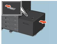
**2** Open the feeder cover of the Large Capacity Feeder on the right.
