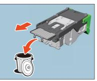
**5** Holding the knob, raise the guide, and return it to its original position.
