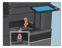
**2** Remove the misfed paper inside the Bridge Unit.
