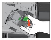
**3** Take the empty staple case out of the staple cartridge. Pull up the empty staple case while pushing both sides as shown in the figure.
