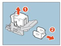
5 Fit the new staple case into the staple cartridge. Insert it to the rear until it clicks.
