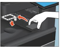
Placing the paper exit stopper back in its original location
