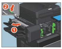
While holding the green lever, open the Hole Punch Unit to remove the misfed paper.
