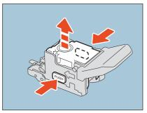
**4** After the transparent cover is lifted, take the empty staple case out of the cartridge.
