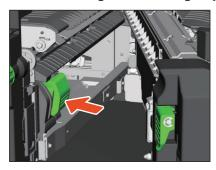
**10** Return the Hole Punch Unit to its original position.
