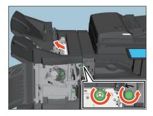
Be sure to turn the knob to the direction indicated by the arrow to remove the misfed paper. If you pull out the paper forcibly without turning the knob, this may tear the paper.
