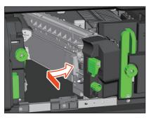
**7** Return the Hole Punch Unit to its original position.
