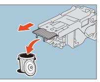
**7** Holding the knob, raise the guide, and return it to its original position.
