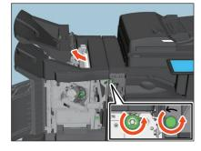
Be sure to turn the knob to the direction indicated by the arrow to remove the misfed paper. If you pull out the paper forcibly without turning the knob, this may tear the paper.
