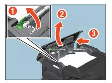
**4** Remove the misfed originals under the feed roller unit.
