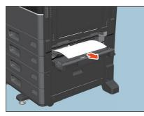
If the paper is misfed on the cover side, remove it as shown in the figure below.
