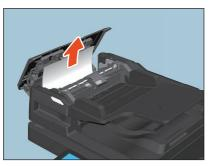
**3** If it is not easy to remove the misfed originals under the feed roller unit, take it off.
