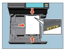
In particular, be sure that the upper limit for thick paper is not exceeded when placing thick paper in the first drawer of the e-STUDIO2020AC/2520AC/2021AC/2521AC. The amount of thick paper you can load in the drawer is lower than that for plain paper.
