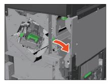
**4** Raise the lever and open the upper receiving tray of the finisher.
