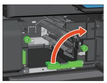
6 When the Hole Punch Unit is installed and used for punching holes, while pulling the green dial toward you, turn it to align the yellow marks on the parts.
