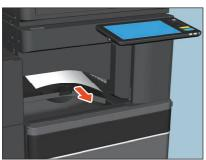
7 If the paper size is small, turn the knob shown in the following figures to send the paper, and then remove the misfed paper.
