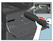
8 Carefully pull the cleaner out until it comes to a stop, and then carefully reinsert it straight into its original position. Repeat this step a couple of times.
