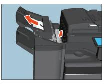
**3** Open the cover holding the handle of the Bridge Unit. When the Hole Punch Unit is installed, proceed to step 5.
