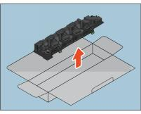
5 Put the used waste toner box in the plastic bag and seal it with adhesive tape.
