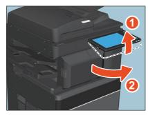
2 While holding the green lever, move the finisher to the left until it stops.
