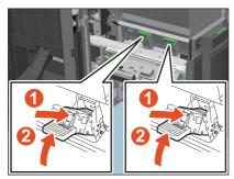
**9** Return the Saddle Stitch unit to its original position. Close the front cover of the finisher.
