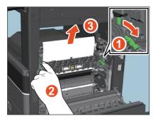
**A** Remove the paper from the exit section.
