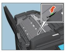
**4** Raise the green lever under the transport guide, and remove the original under the guide plate.
