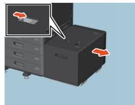
**2** Open the feeder cover of the Paper Feed Pedestal on the right.
