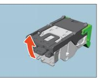
6 Remove the staples if they have fallen between the staple cartridge and the staple case or in the staple receiver.
