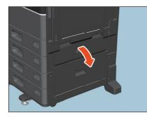
**3** Remove the misfed paper from the drawer and close the feeder cover.
