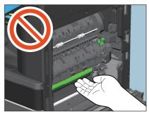
2 Lower the green lever, open the reverse cover and remove the original.
