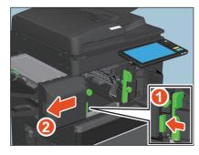
**3 Pull down the green lever on the right-hand unit of the finisher.** The paper exit of the equipment opens.
