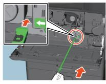
8 Insert the cleaner all the way in, and then pull it back out. For monochromatic models, repeat this 3 times. For color models, repeat this 3 times for each unit. For color models
