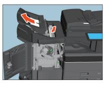
**5** Open the cover holding the handle of the Bridge Unit.
