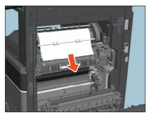
**3** While holding the green lever, remove the misfed paper.
