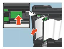
**3** Turn the inner green dial and remove the misfed original.
