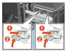
**7** Return the Saddle Stitch unit to its original position. Close the front cover of the finisher.
