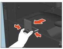
Installing the paper exit stopper in the designated location for improving paper exit
