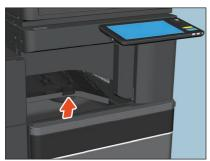
8 For e-STUDIO2020AC/2520AC/2021AC/2521AC and e-STUDIO2525AC/3025AC/3525AC/4525AC, return the two green fuser pressure release levers to their original position.
